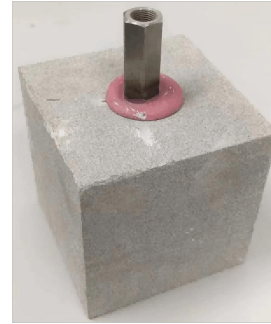
Fig. 1. Rock sample for the physical model experiment of true triaxial hydraulic fracturing.
